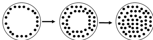
Fig. 6. A schematic showing the development of EPR phases in the iPP particle during the second stage copolymerization.
